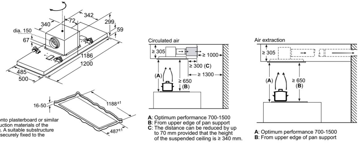
Never fit directly onto plasterboard or similar lightweight construction materials of the suspended ceiling. A suitable substructure is required that is securely fixed to the concrete ceiling.
