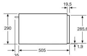
Ovens with an appliance height of 595 mm can be installed above a warming drawer. An intermediate floor is not required.
