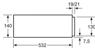
Compact ovens with an appliance height of 455 mm can be installed above a warming drawer. An intermediate floor is not required.
