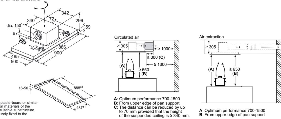
Never fit directly onto plasterboard or similar lightweight construction materials of the suspended ceiling. A suitable substructure is required that is securely fixed to the concrete ceiling.
