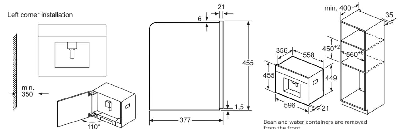
Bean and water containers are removed from the front. Recommended installation height 95-145cm.
