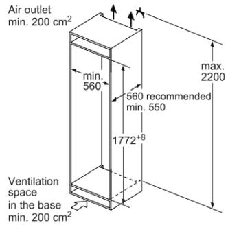
The specified unit door dimensions are valid for a door gap of 4 mm.
