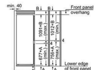
The specified unit door dimensions are valid for a door gap of 4 mm.
