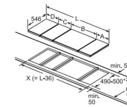
When installing several elements side by side, several assembly kits are also required (Z9914X0).
